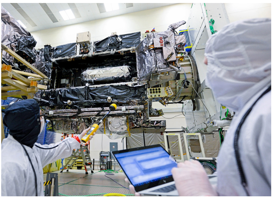
GOES-T undergoes EMI/EMC testing. Credit: Lockheed Martin
